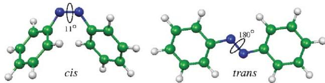
FIG. 1. Structure of trans and cis isomers of azobenzene. The circles highlight the CNNC dihedral angles.
